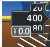
Altimeter displaying ground line
