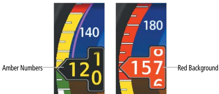
Airspeed Indicator (Approaching and Exceeding V_{NE} )
